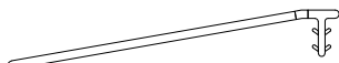
V112 HINGED VINYL NAILING FIN-SIDE - For use at side jambs and sill for Bow and Bay assemblies
