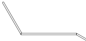
V226 DRIP CAP - VINYL - For use at Head Jamb. Optional for Ultimate Wood Round Top units
