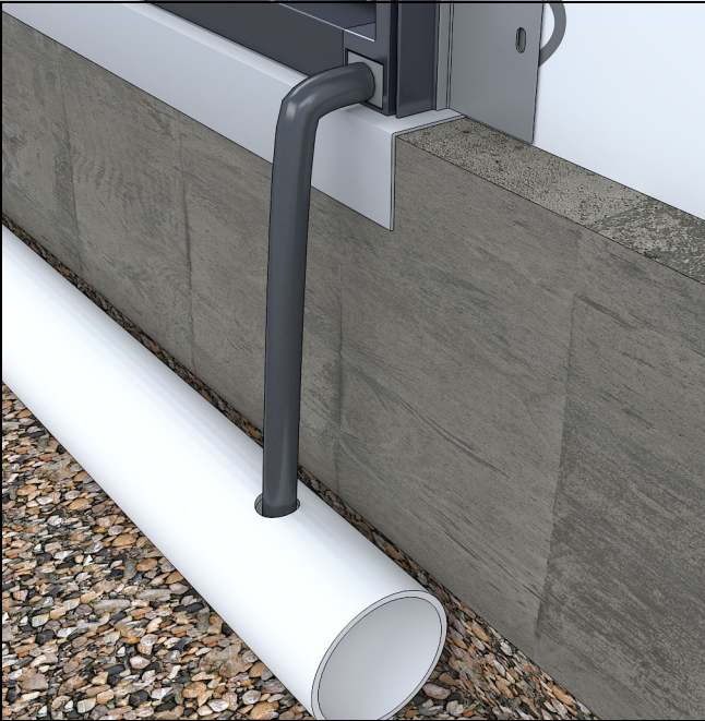
Figure 7 Weep tube terminating into drainage pipe
