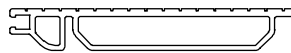
Sill Cover, Spliced Includes: Pile weather strip and end caps Note: Available in LH or RH configurations.
