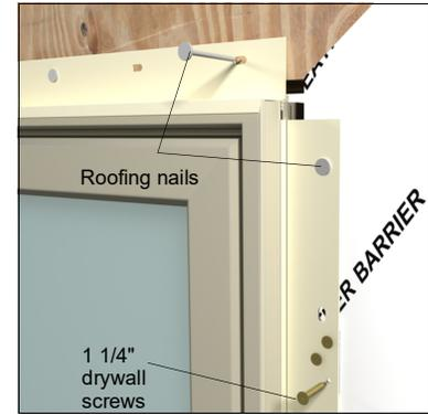
1. Install clips at the recommended locations as shown at the beginning of this instruction. Place the short end of the bracket on the back side of the nailing fin. Attach the clips to the wood jamb liner with the three #7x 5/8" screws provided.
