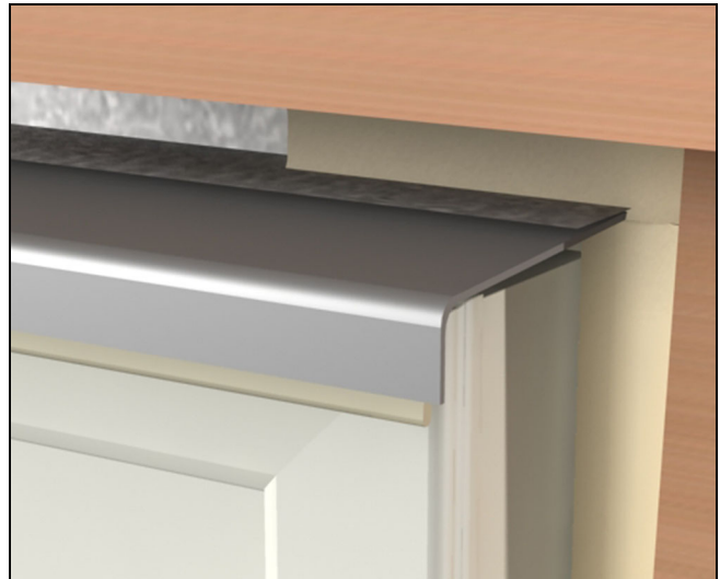
Figure 25 Apply sealant between window and exterior finish.
