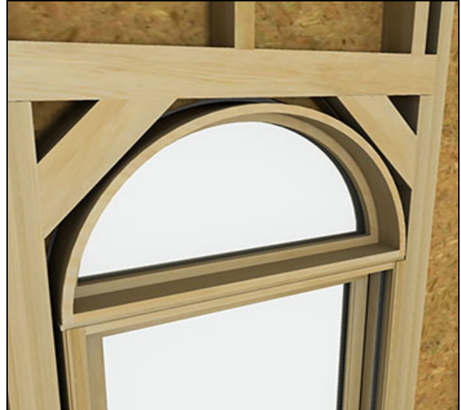
Figure 2 Typical rough opening.
