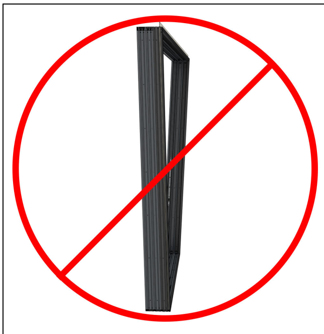
Figure 61 Make sure the entire frame is on the same plane and not twisted.
