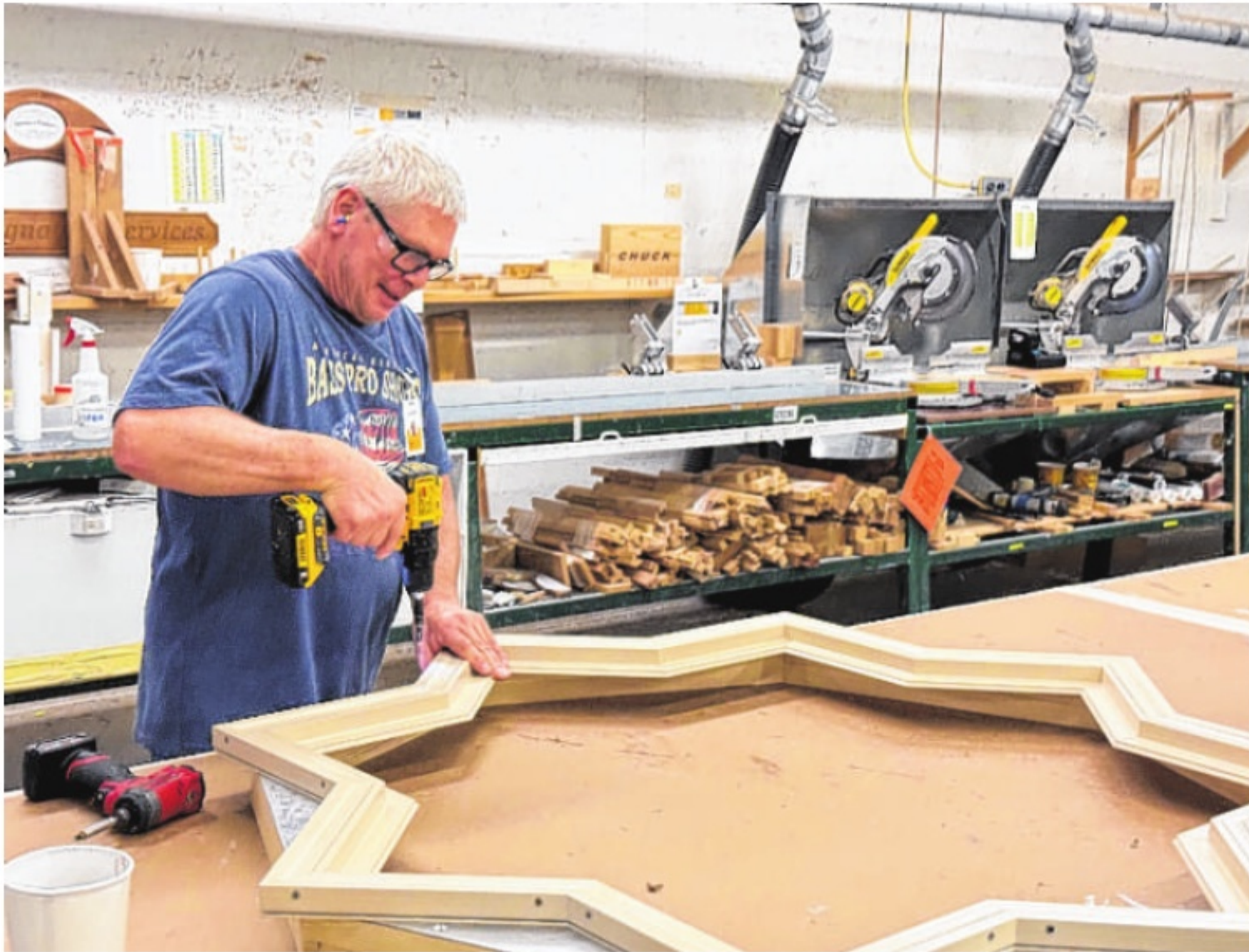
Scott Kimble drills a frame of a star-shaped window at the Marvin factory in Warroad. Marvin specializes in built-to-order custom windows.
