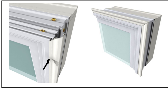
Figure 1: Pressing on the J-Channel
