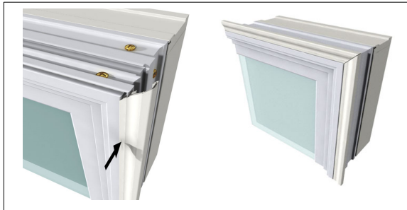
Figure 1: Pressing on the J-Channel
