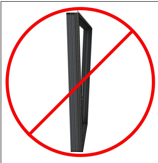
Figure 65 Make sure the entire frame is on the same plane and not twisted.
