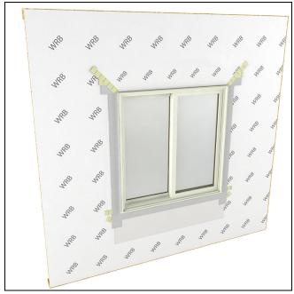
Figure 42 Sealing the Installation in air barrier applications.
