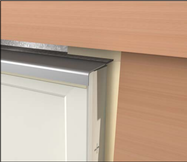
Figure 21 Apply perimeter sealant between window and exterior finish.
