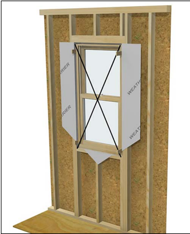
Figure 16 Attaching window with masonry clips or installation brackets.
