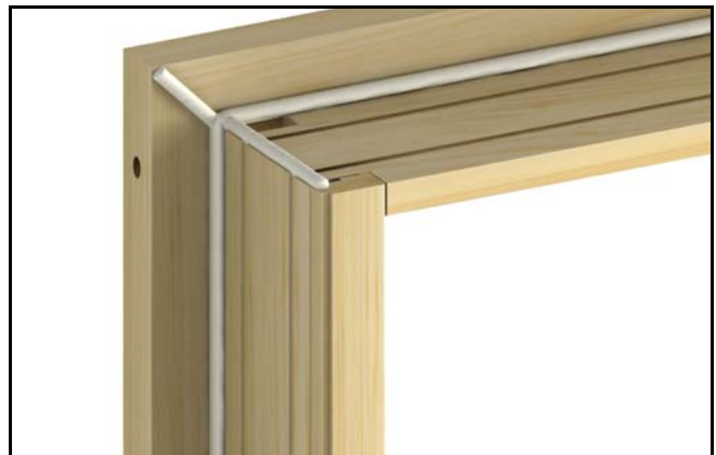
Figure 11 Seal casing joints
