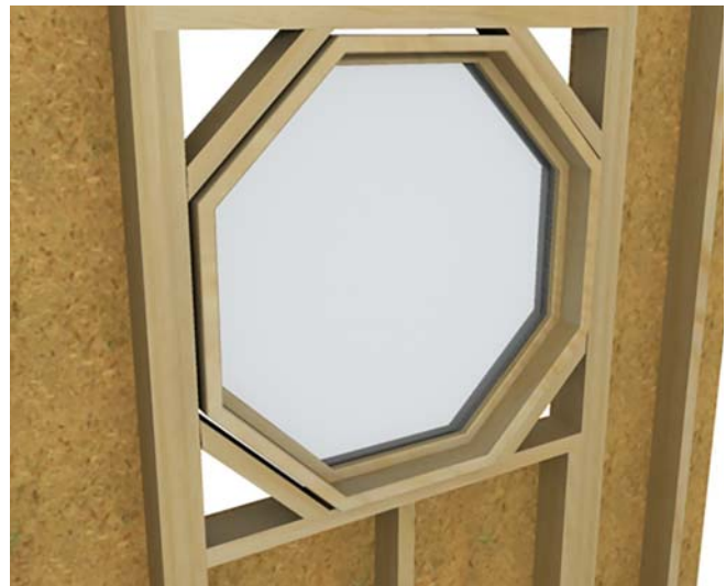
Figure 2 Typical rough opening for octagon.
