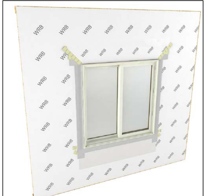
Figure 19 Sealing the Installation in air barrier applications.
