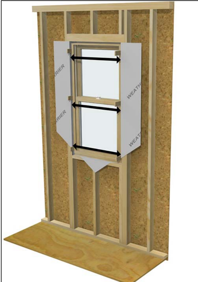
Figure 18 Measure at 3 points and adjust shims until equal.
