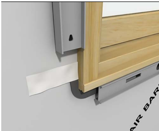
Figure 13 Leveling window, use shims if necessary
