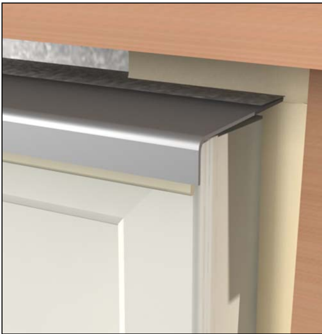
Figure 23 Apply sealant between window and exterior finish.
