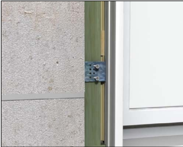
Figure 17 Attaching window with structural brackets.
