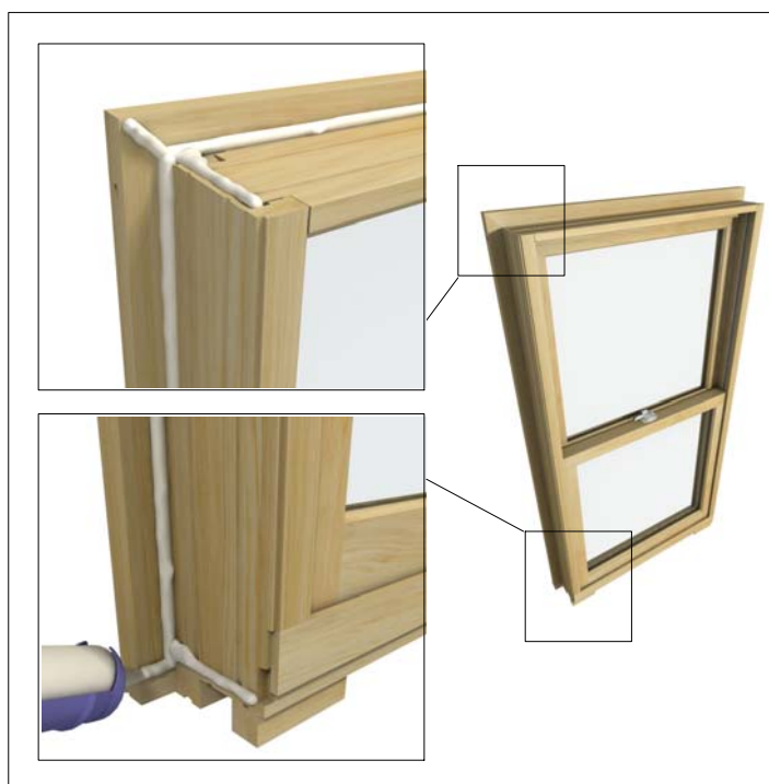
Figure 5: Apply back-caulking to BMC.
