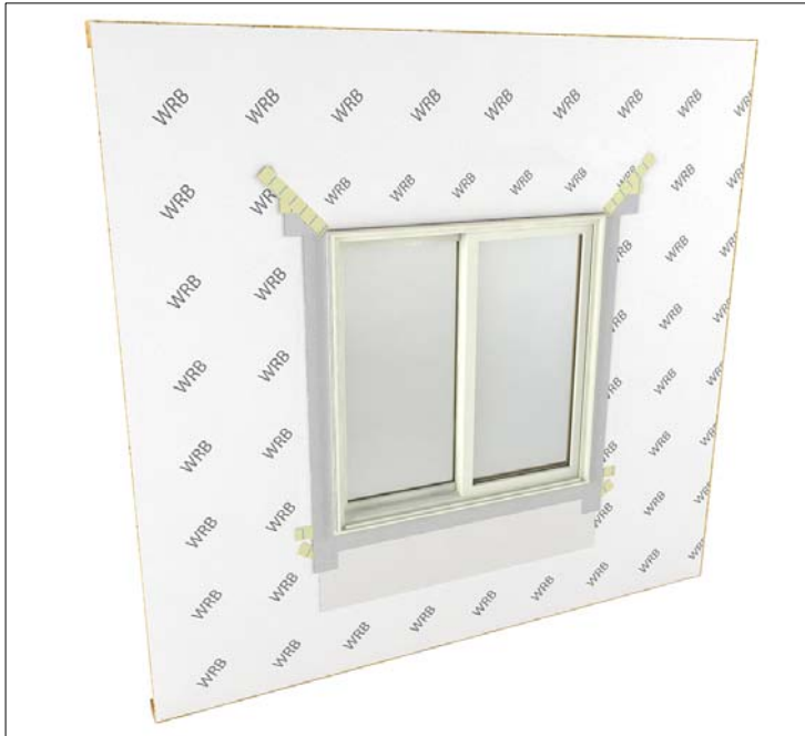
Figure 13: Sealing the installation in air barrier applications.
