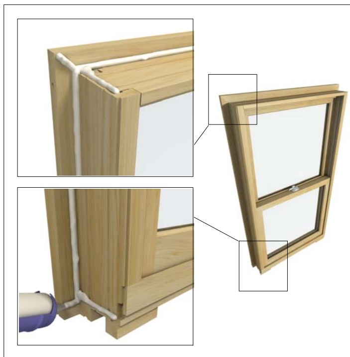
Figure 5: Apply back-caulking to BMC.
