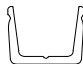
A2810 Stationary Sill Bracket – XOX, Shoe Reinforcement Leveling Block, and Stationary Panel Leveling Block
