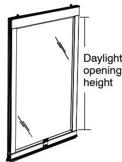
Top Sash Interior View
