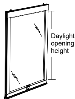
Top Sash Interior View
