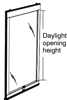
Top Sash Interior View
