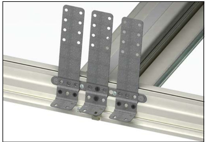
Figure 14 Jamb/Head Jamb bracket placement
