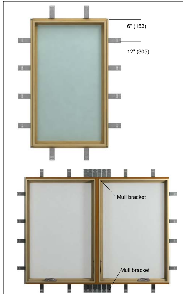
Figure 4 Attach structural brackets and structural mull brackets to frame (ICA frame shown)
