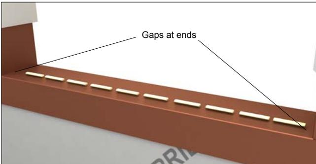
Figure 6 Discontinuous bead of sealant.
