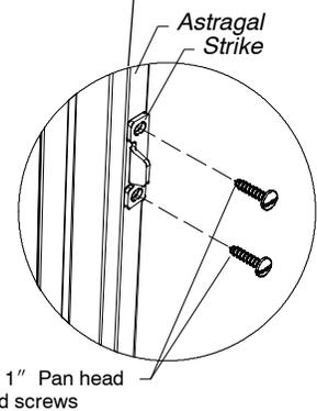
3. Install strike on parting stop, mullion post or astragal (depending on configuration) using #8x1" pan head wood screws as shown in illustration 5. Do not over tighten.
