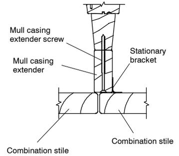
4. Place stationary panel into frame hold in place. Stationary panel brackets are to be installed 6" (152) from head jamb and sill and one at center on each stile. Hold the short side of the bracket against the combination panel and mark the holes on the stile. See illustration 5. Repeat at each location, remove combination panel. Apply stationary brackets to panel(s) using #7 x 3/4" Phillips head screws as shown in illustration 5.
