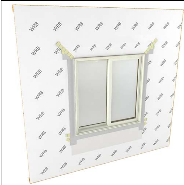
Figure 18 Sealing the Installation in air barrier applications.
