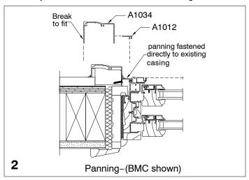
Break lines are provided on the panning components and may be used as a guide for cutting on a table saw or brake. See figure 3.
