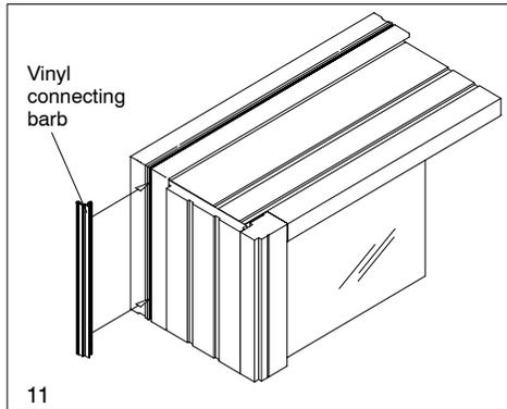
14. Position jamb casings onto the frame kerf and connecting barb ensuring the end of jamb is flush against subsill (or even with sill on door products). Carefully press jamb CBMC into connecting barb and kerf by hand then secure with a rubber mallet. **CAUTION: Do not force if binding occurs as damage may result to the frame and brick mould casing.**
