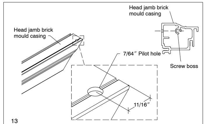
17. Carefully press head jamb CBMC into connecting barb and kerf by hand then secure with a rubber mallet. Again, do not force CBMC onto frame if binding occurs as damage may result to the frame and brick mould casing. Secure head jamb to jamb CBMC with two #8 x 1 1/2" flat head screws provided. See illustration 14.
