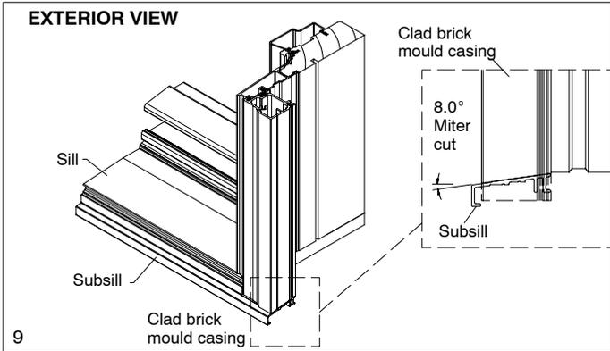
11. Lay one of the casings along the jamb kerf ensuring the bottom is snug against the subsill of the window product or flush with the sill on door products.
