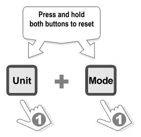
When an error is noted in the operation of the motor unit (indicated by a <u>Flashing RED light</u> on the wall plate or status indicator), the unit can be "Reset" by forcing a re-initialization via the remote control.
