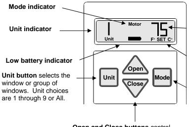
Open and Close buttons control windows or blinds. They will also stop the window or blind in a partial open position by pressing the button opposite window or blind travel Room temperature with measurement system (F° or C°) indicated below
