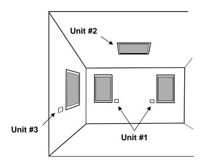
In this illustration the two front windows are set to "Unit" #1. This allows the home owner to operate both windows with one command sequence from the remote. The side window and skylight are assigned their own "Unit" numbers. This allows each of these units to be controlled individually.
