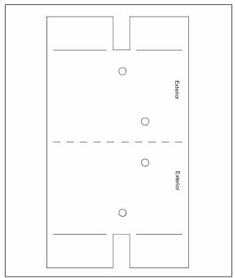
NOTE: The template must line up on either side of the sash pivot pin grooves. Make sure to note interior and exterior edges of the template which correspond to the interior and exterior sides of the sash.
