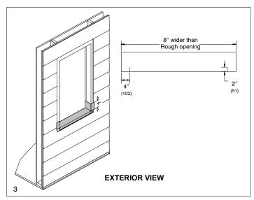
NOTE: If metal or PVC pan sill flashing is to be used, install now.
