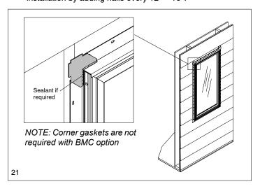
**IMPORTANT:** Marvin nailing fin is not designed to be a waterproof flashing.
