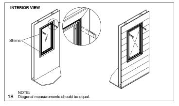
NOTE: Proper shimming is extremely important. Over or under shimming will result in bowed jambs and/or head jamb. Be careful not to bow the jambs.
