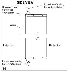
NOTE: It may be necessary to trim nailing fin to fit within existing openings.
