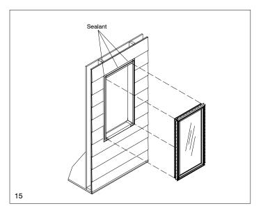
Center the unit or assembly into the rough opening. Check the unit for level and plumb. If required, place shims along the sill to level. See illustration 16.
