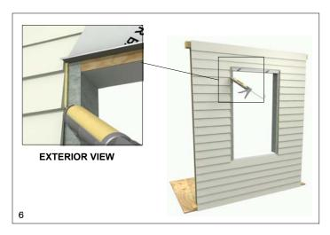
7. Tool sealant ensuring siding gaps are sealed. Apply a bead of sealant across the ends and length of the drip cap. Apply a continuous bead of sealant (see recommended sealant on page 1) across the top and sides of the window opening. Apply sealant to rough opening bottom leaving a 2" gap at each corner. See illustration 7. Proceed to Installing the Unit section.
