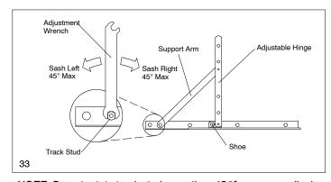
NOTE: Do not rotate track stud more than 45° from perpendicular in either direction.
