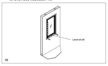
14. When sill is level in opening, tack both bottom corners of the jamb nailing fin to the sheathing. DO NOT drive the nails all the way in at this time. See illustration 17. Be sure to plumb vertically (interior to exterior) at side jambs, then tack top corners as well.
