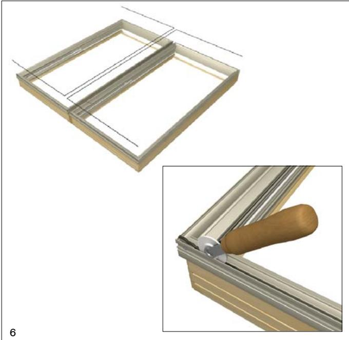
9. Measure the width of the mullled assembly at cladding (distance perpendicular to the mull). Subtract 5/32" (4) and cut two pieces of outside frame trim (A148) to adjusted measurement using a hacksaw or power miter saw.
