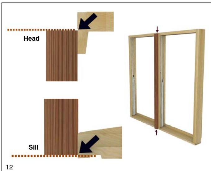
16. Measure width of the unit plus width of exterior casing and cut and notch subsill to length. Treat any cut parts with a water repellent wood preservative. Apply sealant next to the kerf on the subsill and secure subsill to sill with #8-15 x 1 3/4" wood screws placed per illustration 13.
