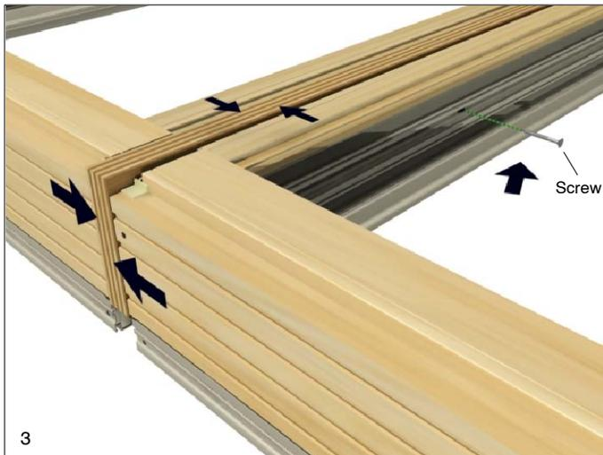
5. Mull the interior with 1/2" x 5/8" crown staples 2" (51) from each end and spaced every 3-5" (76-127). Complete this step by stapling three staples into each unit at the sill and header mull joint. See illustration 4.
