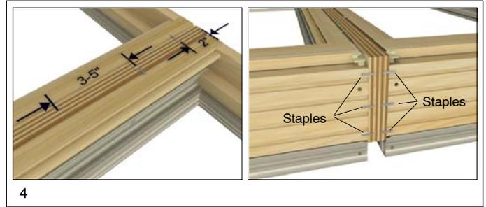
6. Turn the unit over and apply the exterior mull casing per the following exterior space mull instructions for Clad Units; for Wood units proceed to step 14.
