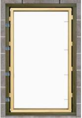
Insert packing at 400mm intervals and fix at each packing location
