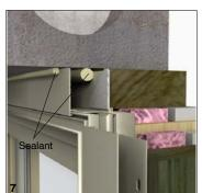
A range of aluminium frame expanders are available for integrating windows to structures.
