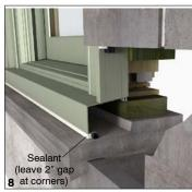
An optional range of decorative aluminium exterior casings and sills in traditional profiles are available for integrating windows to structures.
