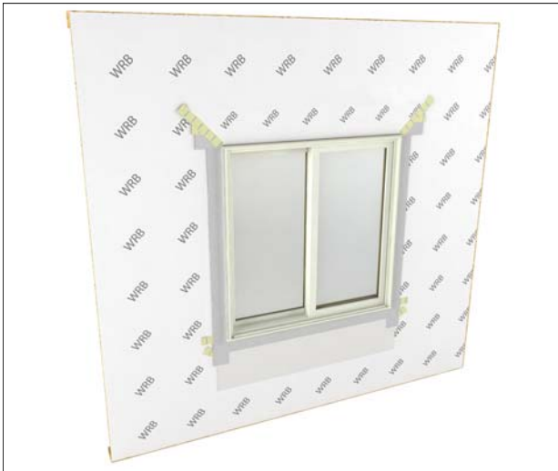
Figure 10 Sealing the Installation in air barrier applications.
