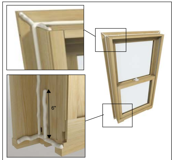
Figure 6 Seal casing joints (brick mould casing showing).
