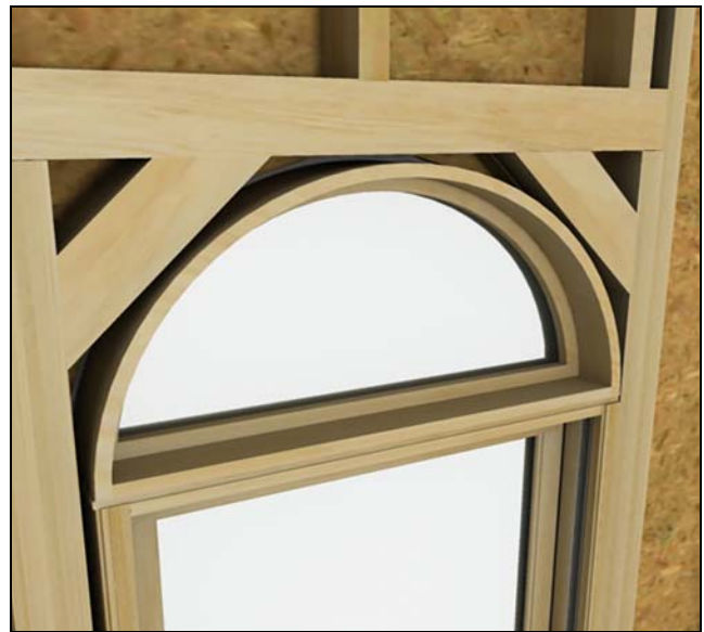
Figure 2 Typical rough opening.
