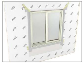
Figure 11 Flashing the installation
