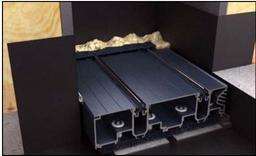
Pocket with open face slot in concrete with a 2 3/8" (60) slot recess leaving 0" available floor thickness. The concrete is the finished floor and flush with the top of the sill.
