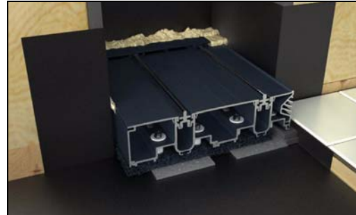
Pocket application of open face slot in wood construction showing 1" (25) slot recess. Available flooring is 1 3/8" (35). Flooring used is 1/4" (6) leaving 1 1/8" (29) sill face exposed.
