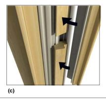
Figure 4: Replacing Jamb Fillers
