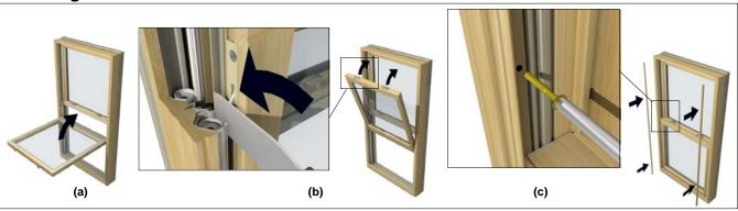
Figure 8: Installing Bottom Sash
