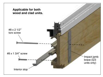
Figure 9: Predrilling the impact jamb brace.
