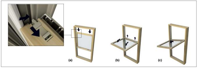
Figure 6: Removing Top Sash
