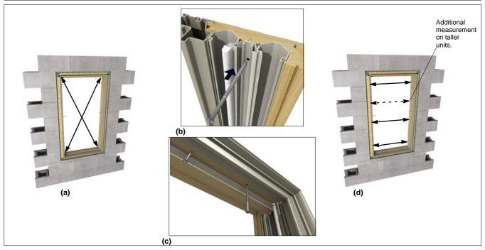
Figure 10: Using the jamb adjustment system
