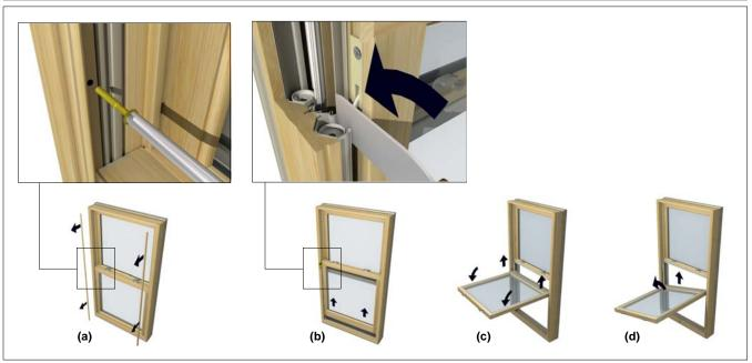
Figure 5: Removing Bottom Sash
