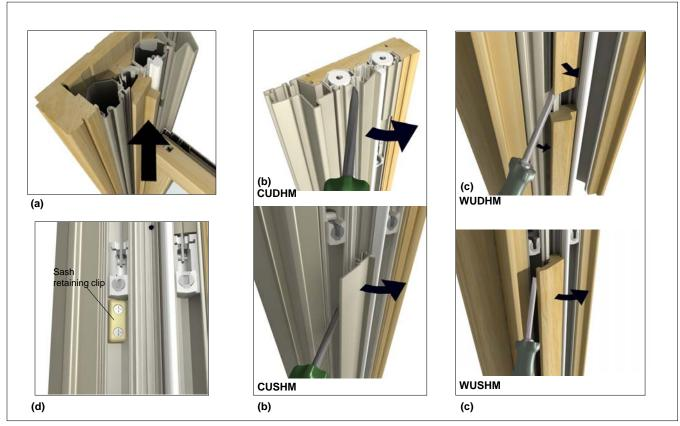
Figure 3: Removing Jamb Fillers
