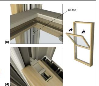
Figure 7: Installing Sash
