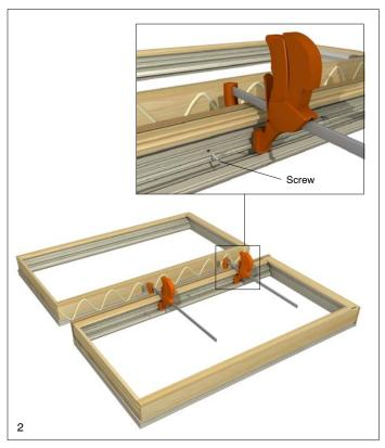
4. Remove clamps and place the units together making sure the frames are even and flush at the sill. Fasten the unit to the mull filler through the predrilled holes in the jamb liner with the supplied mull screws as described in the preceding step. See
