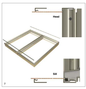
11. Run a 1/4" (6) bead of sealant/adhesive on top of mull blocking at edge of mull and sides approximately 2 1/2" (64) back. Cut appropriate width pieces of foam block and press into adhesive as shown in illustration 7 to both ends of the mull.
