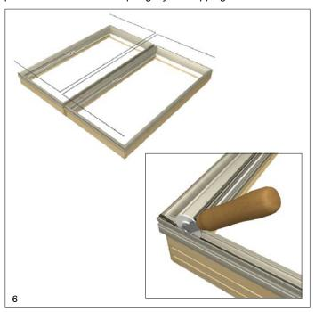
Measure the width of the mulled assembly at cladding (distance perpendicular to the mull). Subtract 5/32" (4) and cut two pieces of outside frame trim (A148) to adjusted measurement using a hacksaw or power miter saw.
