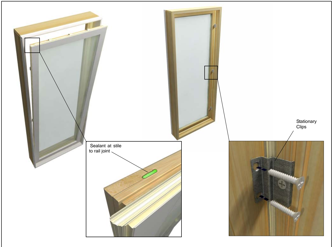
Figure 3 Installing stationary sash and fastening in frame.
