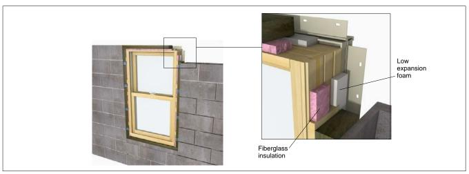
Figure 11: Insulating the rough opening
