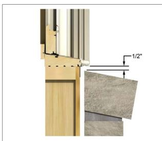
NOTE: On standard wood frame construction with brick veneer, make sure there is at least 1/2" (13) between bottom of window sill (or eventual placement of the window) and the top row of brick to avoid "brick bind".
