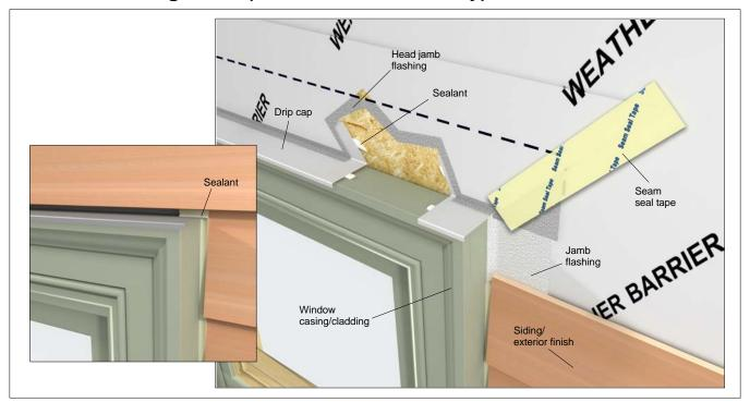
Figure 14: Flashing windows with casing in typical wood frame construction (non recessed masonry).
