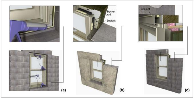
Figure 10: Sealing recessed masonry openings
