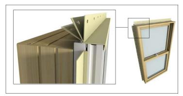
Figure 4: Extend nailing fin.
