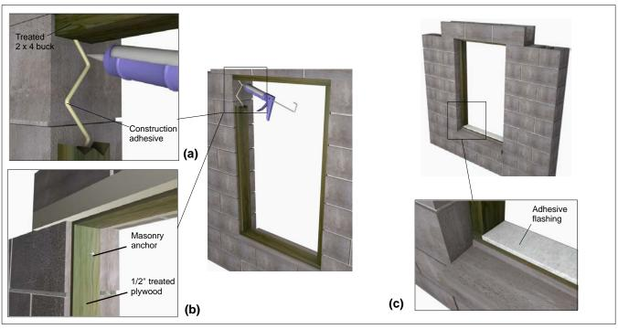
Figure 1: Preparing openings for concrete block openings.
