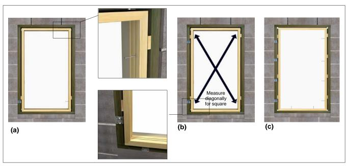
Figure 6: Plumb and square unit. (Illustration shows both structural bracket and jamb screw installation.)
