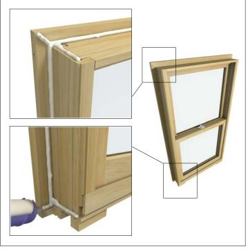
Figure 5: Apply back-caulking to BMC.
