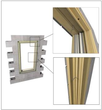
Figure 9: Exterior View, fastening through UDH frames.
