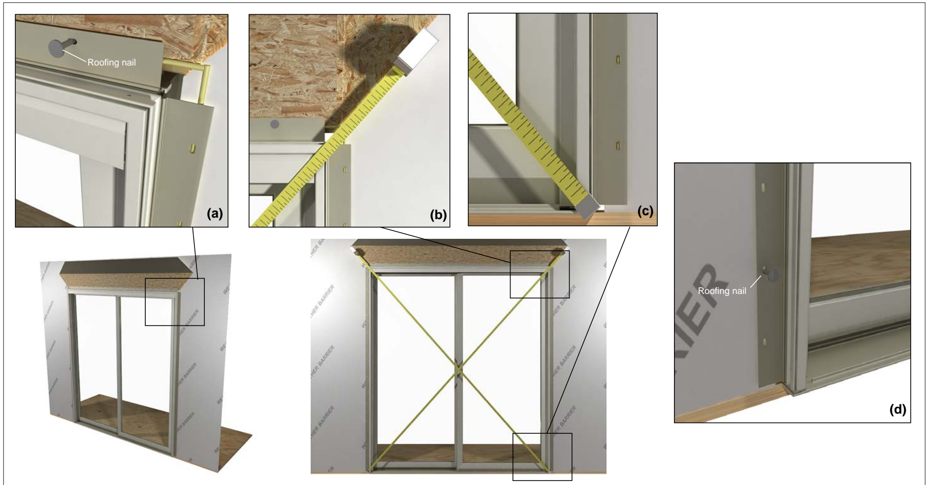
Figure 5 Square the Door to the Sill.
