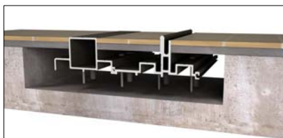
Recessed Sill with Drainage - Stacked
