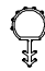
V147 – Weather Strip Sill – UDH-NG, USH-NG, UDHP-NG and UDHT-NG Header – UDHP-NG and UDHT-NG
