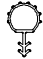
V147 – Sill Weather Strip Bottom Check Rail (BK only) – CUDH-NG, CUSH-NG, CUDHP-NG and CUDHT-NG Header – CUDHP-NG and CUDHT-NG Replaced with V2779
