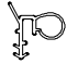
V2403 – Top Check Rail Weather Strip CUDH-NG and CUSH-NG For use on units produced prior to 9/29/2014
