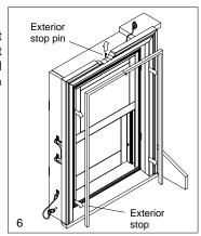
Remove the two frame retainer pins and carefully pull the bottom of the insert out to the exterior to remove unit from frame. See illustration 7.
