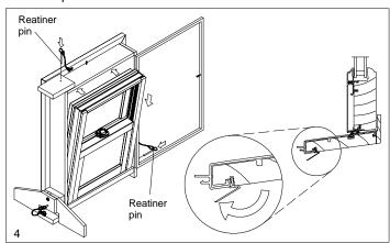
Pull out on the spring loaded interior stop pin and swing the interior stop into place and release the pin. See illustration 5.
