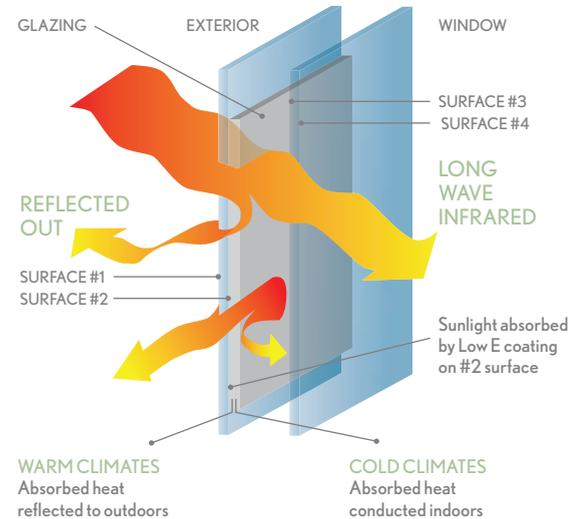
Low emissivity glass features a double metallic coating on the inside glass, which can reflect or absorb the sun's warmth to enhance either heating or cooling while reducing the effects of damaging UV rays.
