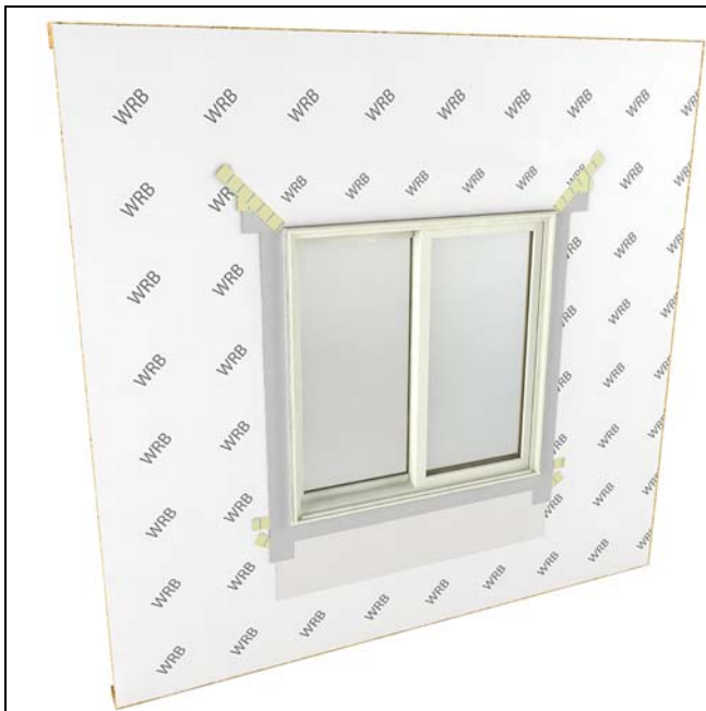
Figure 18 Sealing the Installation in air barrier applications.
