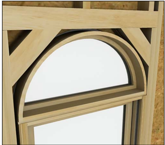
Figure 2 Typical rough opening.
