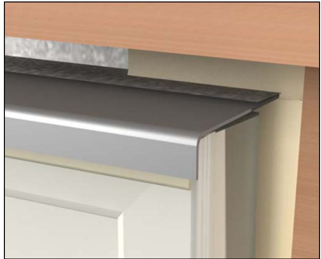
Figure 22 Apply sealant between window and exterior finish.
