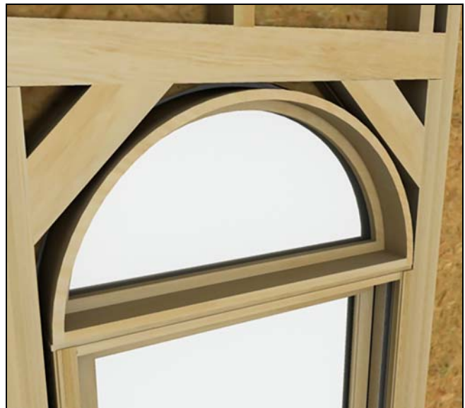
Figure 2 Typical rough opening.
