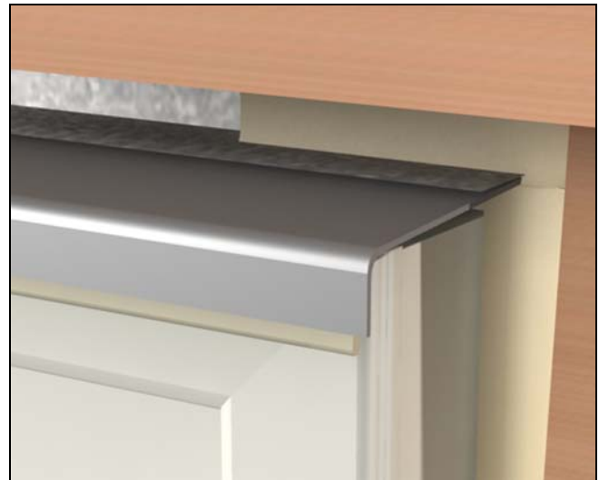
Figure 21 Apply sealant between window and exterior finish.
