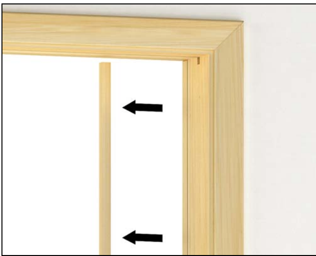
Figure 6 Remove parting stops from side jambs
