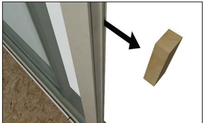
Figure 5 Remove shipping blocks from the operator panel.
