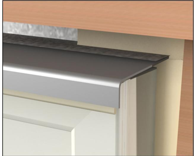
Figure 24 Apply sealant between unit and exterior finish at head jamb.
