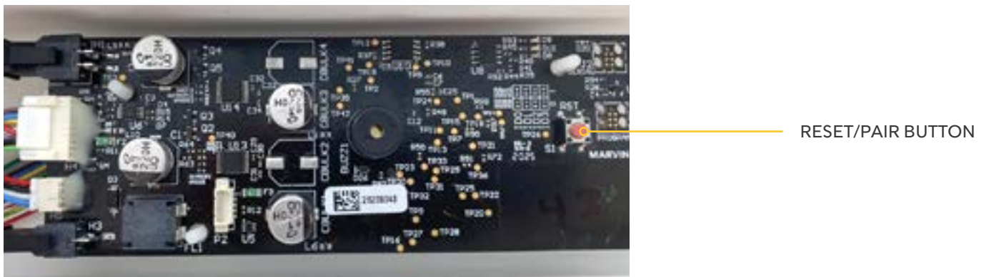
AWAKEN CONTROL BOARD
